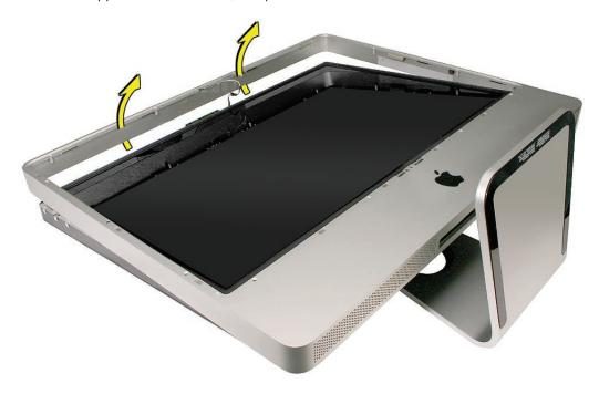
5. Notice the connected microphone cable at the top of the bezel. Without straining the cable, hold the bezel up, and disconnect the microphone cable from the cable extension.
